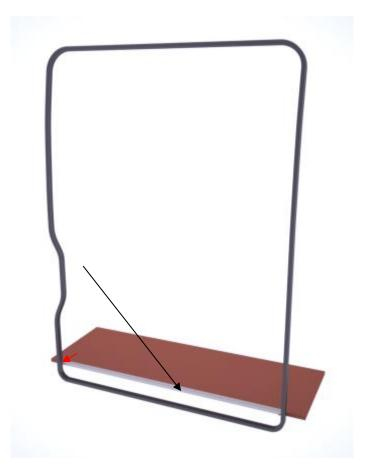
1) Install the bottom profile to the flooring with 4 pcs of 3.5x16mm sunkhead screws. The profile should be installed firmly against the floorboard. The floorboard should be solid wood on the positions of the screws, please check before fixing.
