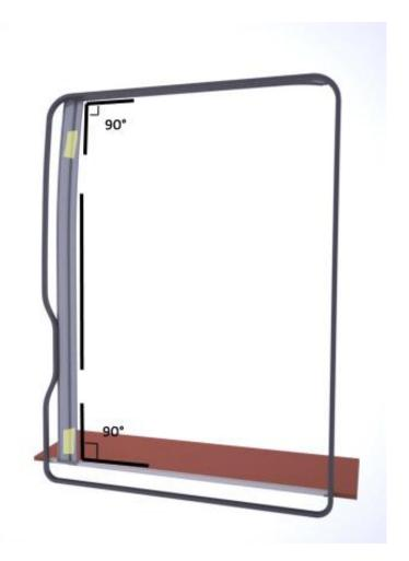
8) Position the bottom side of the cassette and pullbar assembly on the lower profile. It should be easily positioned and excessive force should not be needed. Make sure to leave on the packing tape.
