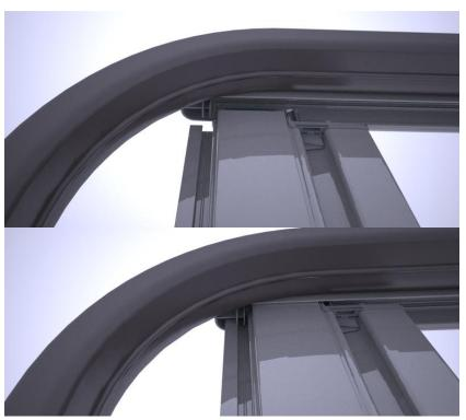
6) Slide the topside of the cassette and pullbar assembly into the slot of the top profile. The cassette and pullbar should be pushed into the topside fully, see lower image.
