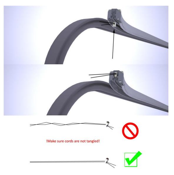
18) Make sure to take out the slack from the cord while fixing the cordtensioner to the cord. Position the topside cordtensioner into the top profile endcap.
