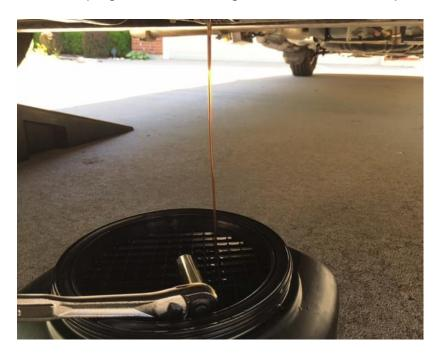
6 – Once the old oil has drained, and you have removed the old Teflon from the drain plug and put new on it, re-install the drain plug.
