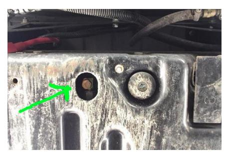
5 - Place the drain pan under the plug, then remove the plug. Very important to use a deep well socket as the plug will fall into the socket. DO NOT attempt to loosen and remove by hand. Use the socket for the entire removal, or you may loose the plug in-between the generator and the skid plate.
