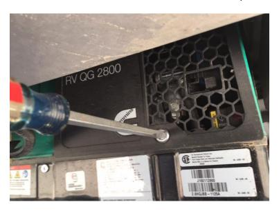
3 – Locate the dipstick (looks just like one on a lawnmower. Small black twist cap) and remove. This is also the fill port.
