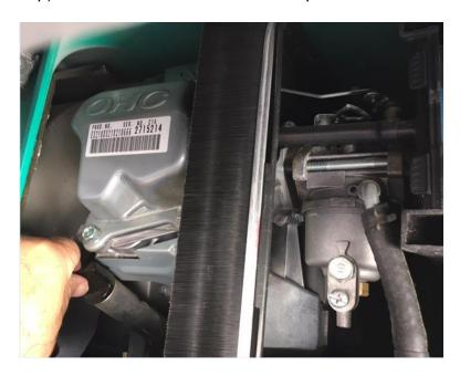
4- Locate oil drain plug (It's a brass bolt head located in a round cut out on the underside of the generator)
