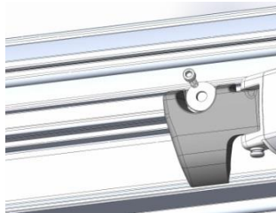
Remove old backing washer
